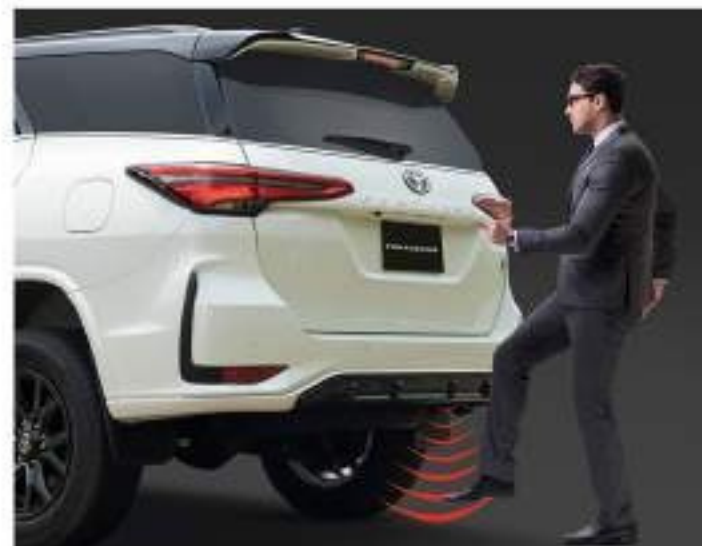
Power Back Door with Kick Sensor Equipped with rear sensors so you can conveniently open the trunk with just a kick of the foot.
